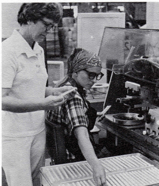
PROCESS CHECK . . . Claudia Perchal (seated) applies a second fill as waterproofing on a 710 connector part, while Arlene Boyd — a process checker — checks her work.
