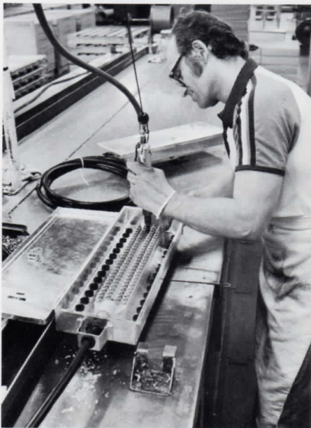
Larry Standley, utility operator, bolts cable terminals to a box and cover assembly.
