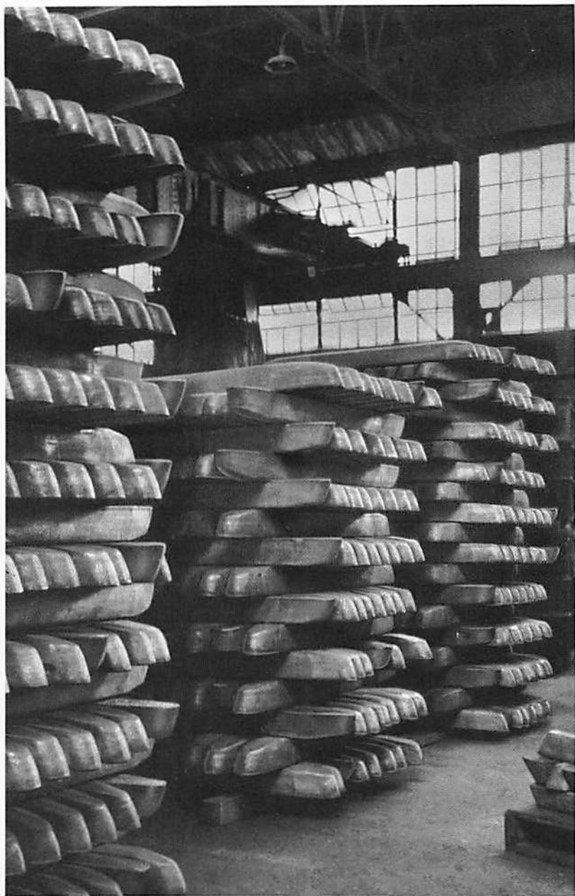
Copper, reclaimed in Nassau's furnaces, will be returned to Western Electric plants, drawn into telephone wire.
