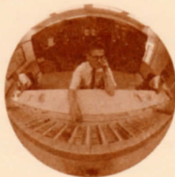
Western Electric-built SCAMA Board at the Goddard Space Flight Center has push-button global conference call capability.
