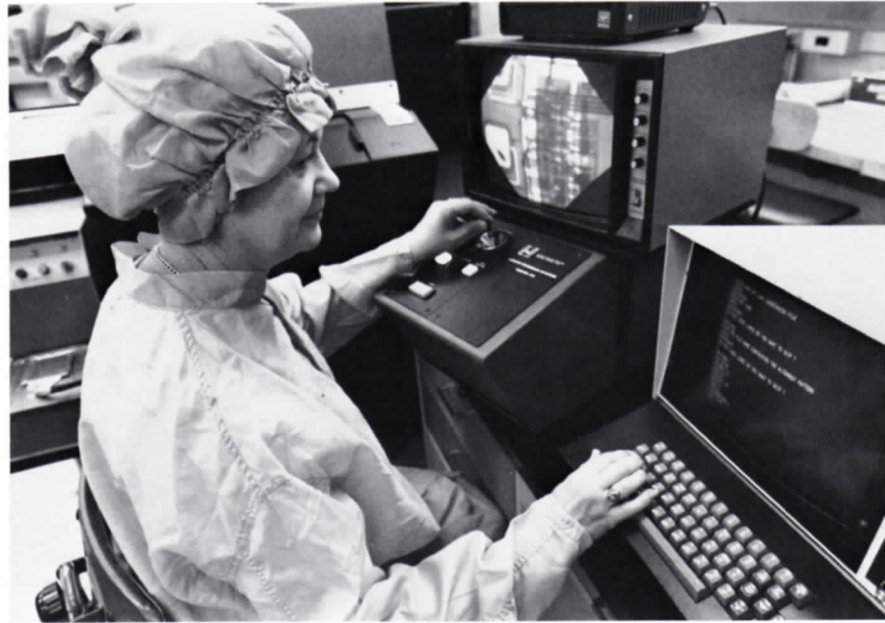
Today —This picture incorporates three new technologies that have had an enormous impact on WE manufacture. The system above uses a computer to control a laser that is trimming a VLSI (very large scale integration) chip.
