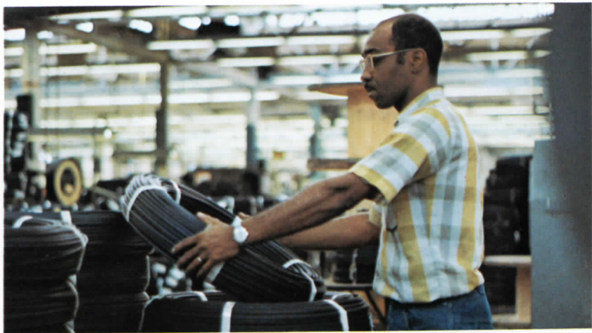
Coiled "C" Drop wire, which connects a customer's telephone to a nearby outside cable, is readied for storage and shipment from the Baltimore Works.
