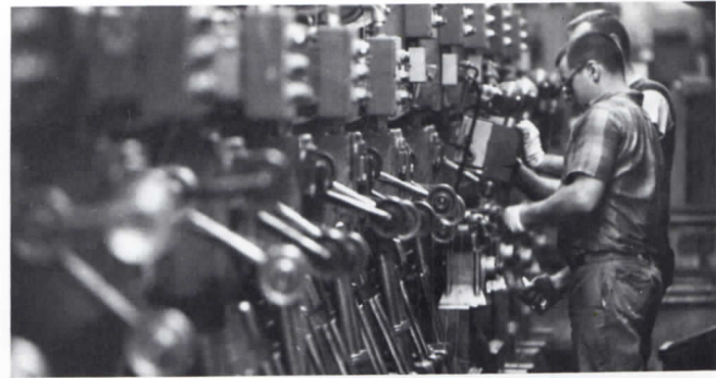
Operator installs single spool containing insulated conductor for twisting. Two conductors are twisted together to minimize "cross talk" during phone calls in finished cable product.
