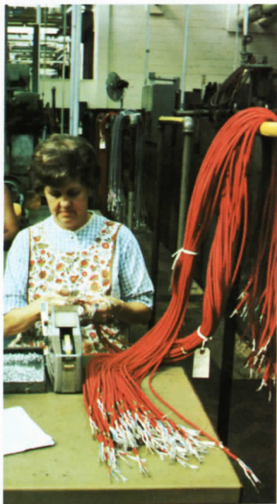
Cord shop employee tapes metal links to prong-shaped connector on switchboard telephone cords.
