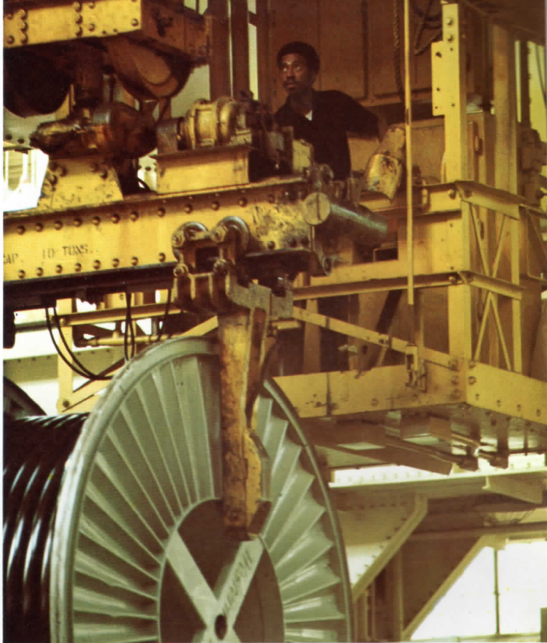
An overhead crane operator positions a reel of telephone cable for shipment from Western Electric's Cable building in Baltimore.
