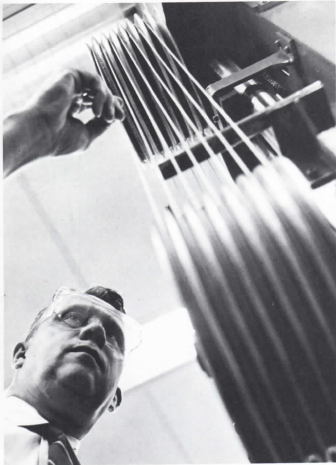
Engineer checks insulation of aluminum conductor wire before it is used in plastic insulated cable.
