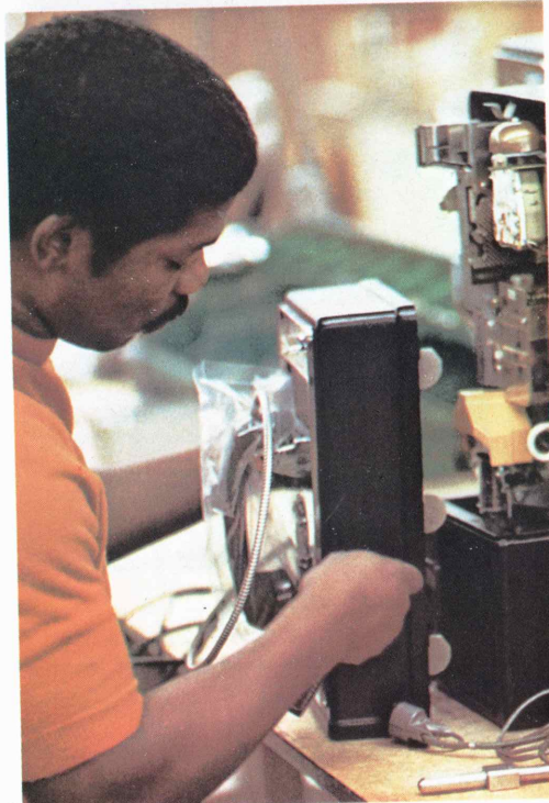
Above: An employee at the Communications Products Center in New York operates a pre-analyzer machine which detects and pinpoints defects in telephone sets that the Bell telephone companies return to WE for refurbishing.
