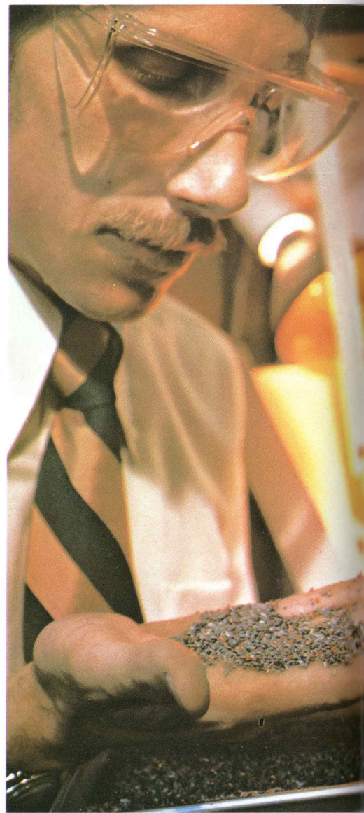
Above: At our Engineering Research Center, an engineer holds pellets of plastic reclaimed from the jackets of telephone wires. The technique for recycling this type of plastic was developed by Western Electric.
