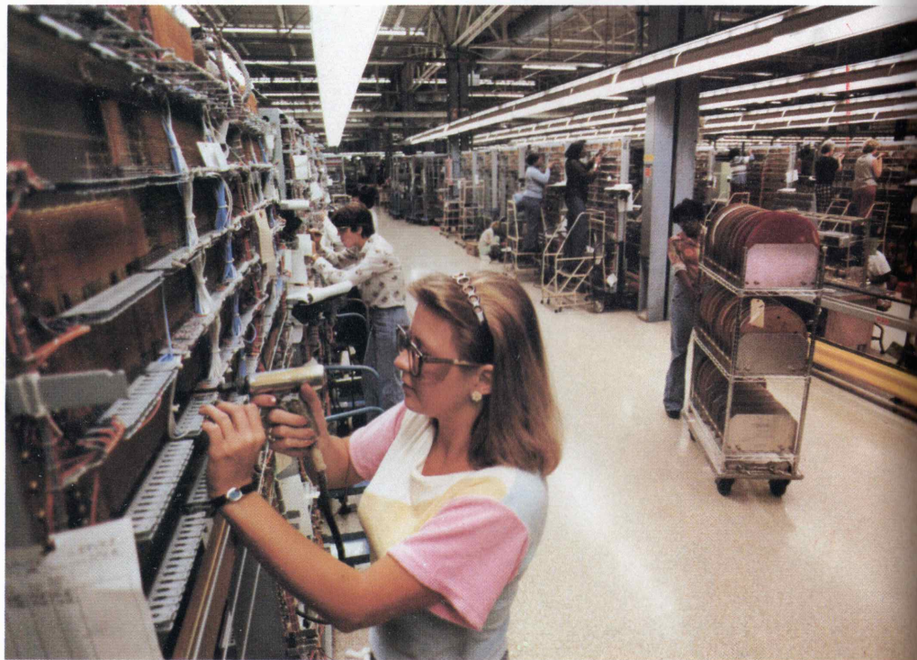
Top: The No. 1 Electronic Switching System (ESS) is manufactured in Dallas. It is designed for big city central offices serving up to 130,000 telephones.
