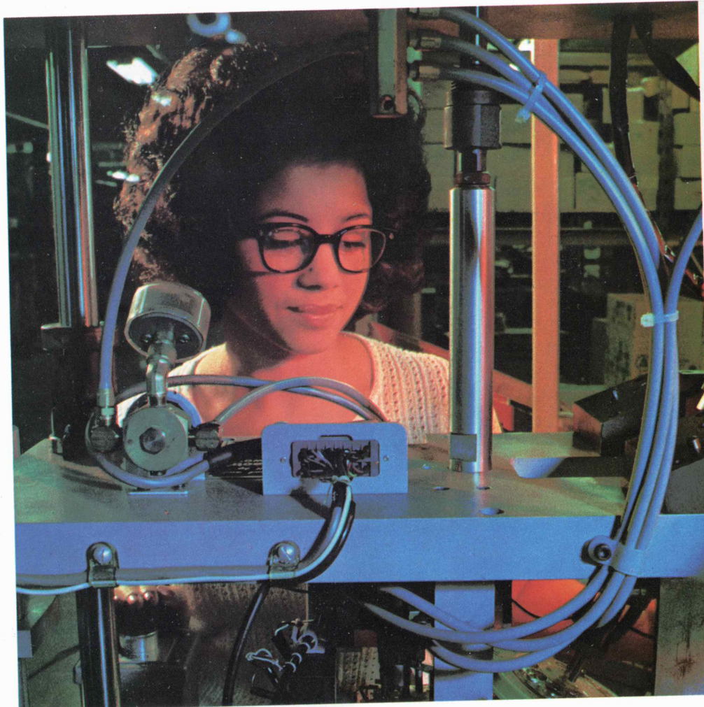
Above: An employee at the Communications Products Center in New York operates a pre-analyzer machine which detects and pinpoints defects in telephone sets that the Bell telephone companies return to WE for refurbishing.
