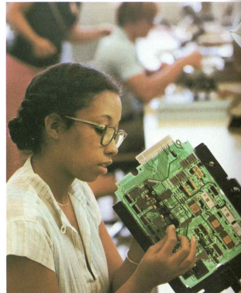
Top Left: An engineer at the Richmond Works examines an artmaster created in two minutes by the Laser Artmaster Generator in rear. The old method took 8 hours.
