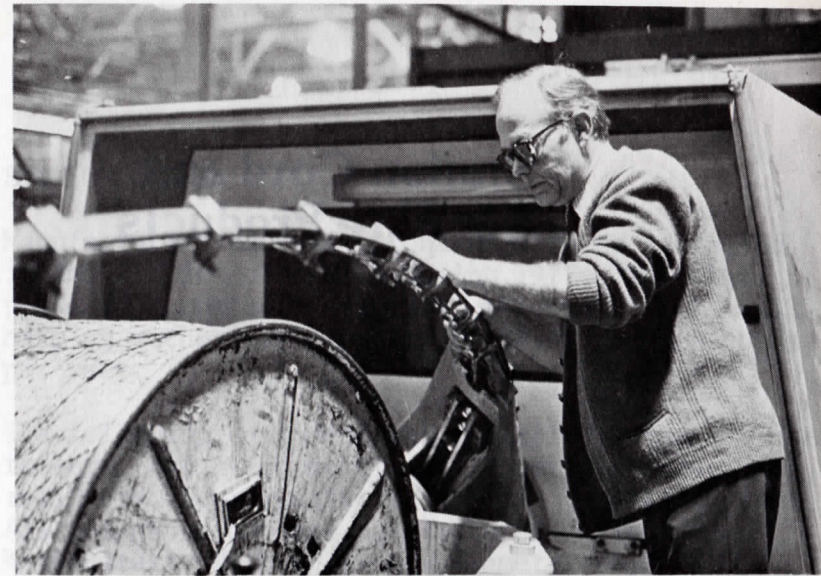
CABLE AND WIRE PRODUCTS: Above - Joe Swenson checks the cable lay at the Northampton strander take-up. Bottom left - Bill Kinsley examines the edge-forming key in steel tape overlap die. Bottom right - Lee Baldauf checks the die string-up on SAMP No. 4 wire drawing machine.
