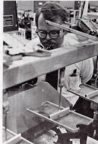
SWITCHING PRODUCTS: Above - Bob Wemhoff watches a shop operator solder the new multi-conductor strapping tape to a small crossbar switch. Bottom left - Bob Douglas is shown with the new laser multi-lead welder in the small crossbar switch area. Bottom right - Marvin Rohwer, Dan Dankoff, and Gary Larson are pictured with the new single comb miniature wire spring relay welder.
