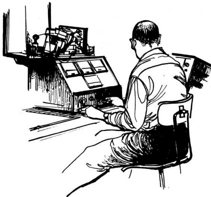
Picturephone display units being assembled and tested at Western Electric's Indianapolis plant. Among the many operations: mounting the picture tube and frame assembly on the ring stand (top left), checking circuit boards visually (top right), placing them in the display unit (bottom left), and finally, testing for picture alignment.
