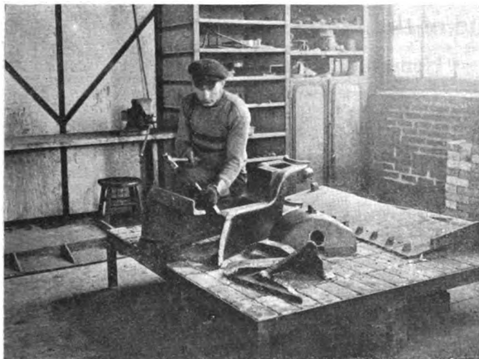
Fig. 1. Chiseling the Break Preparatory to Welding
