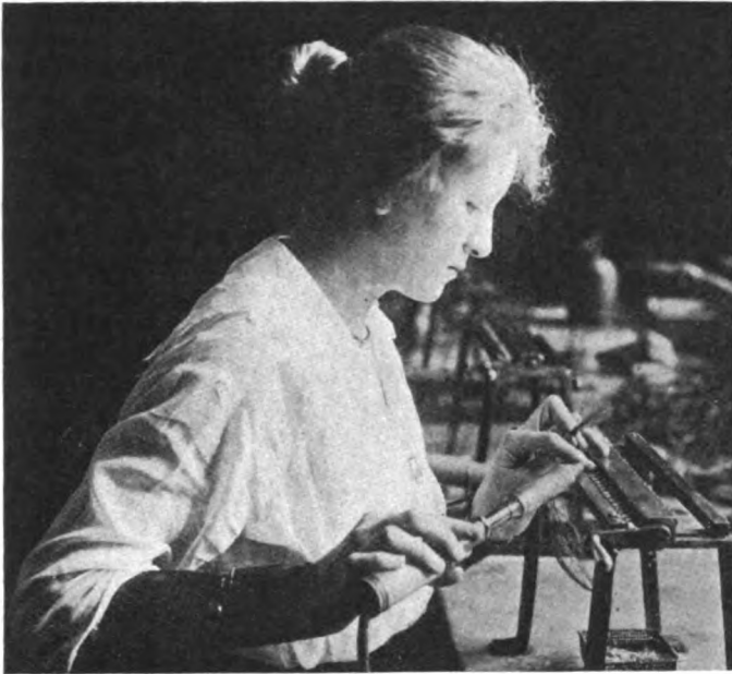
Fig. 1—Soldering the Coil Wire to the Pin and Sleeve Assembly
