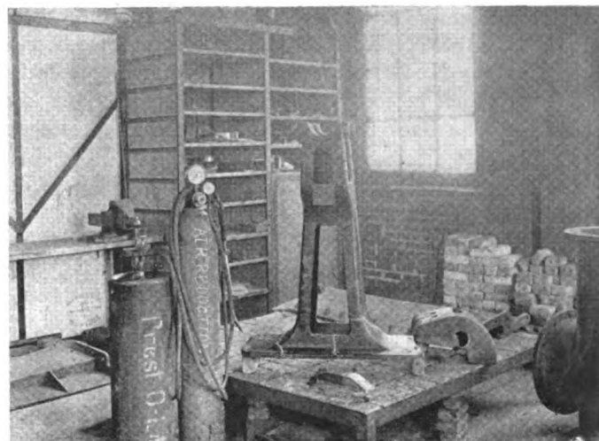
Fig. 3. The Mended Casting, Placed on Two Bricks to Prove Its Strength. The Chalk Marks Show Where the Breaks Were
