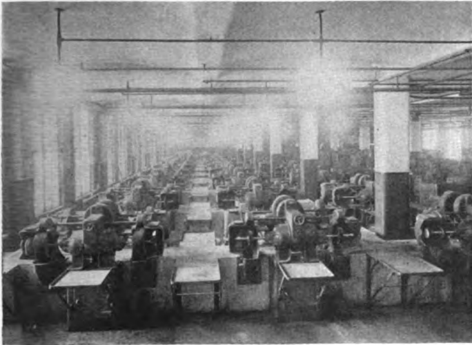
Fig. 4—Buffing Department at Hawthorne Equipped with the New Variable Speed Buffing Motors
