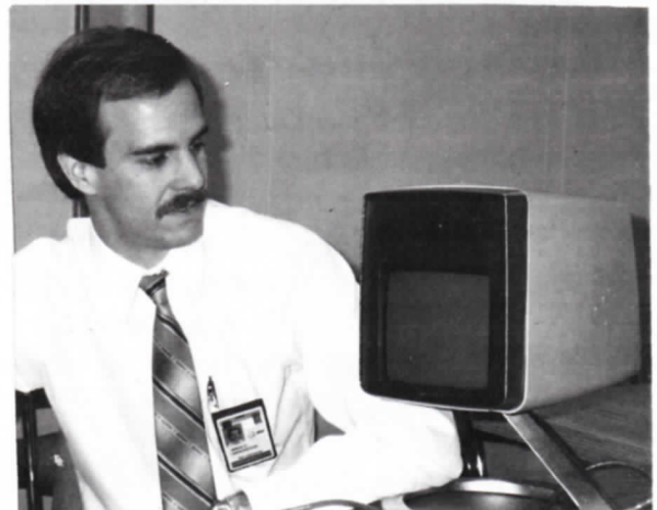
Brian shows the PICTUREPHONE , an early forerunner of video teleconferencing introduced at the World's Fair in New York in 1964. The Picturephone transmitted a semi-moving picture over phone lines. The Picturitel didn't catch on and the project was discontinued in the early 1970s.
