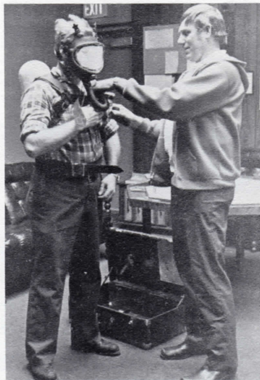
LEAD THE WAY . . . Tramp (right) adjusts a Scott Air Pack on Gulliksen. The device contains oxygen for fighting fire in dense smoke. Paper in the face mask simulates smoky conditions.
