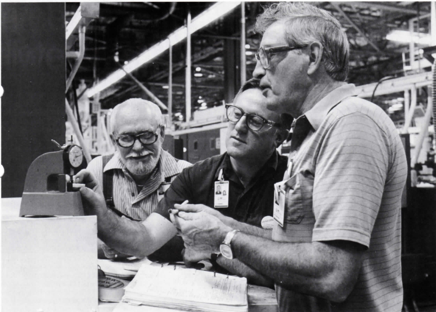
LISTEN CAREFULLY . . . Charlie Patterson (from left) of Dept. 283 and Lentis Campbell of Dept. 087 listen to trainer Bill Huetsen explain how to properly test the thickness of C plenum cable. Listening to directions is critical for employees who work on the jacketing lines in Building 50.
