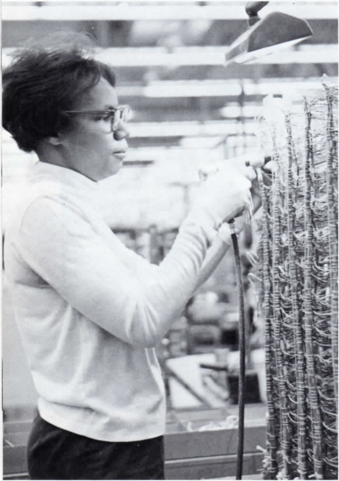
Fay Allen (422) contributes to a quality product as she wires a crossbar unit cable.
