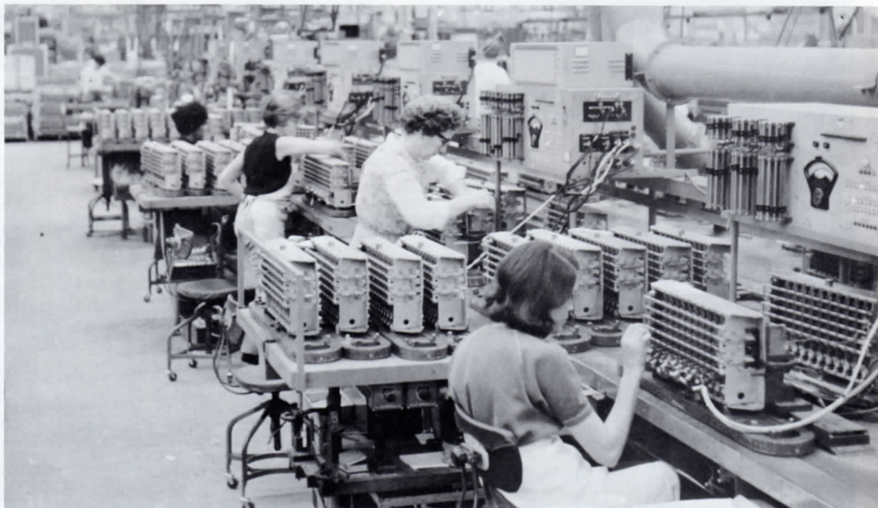
Switch testers in Department 134 check for quality.
