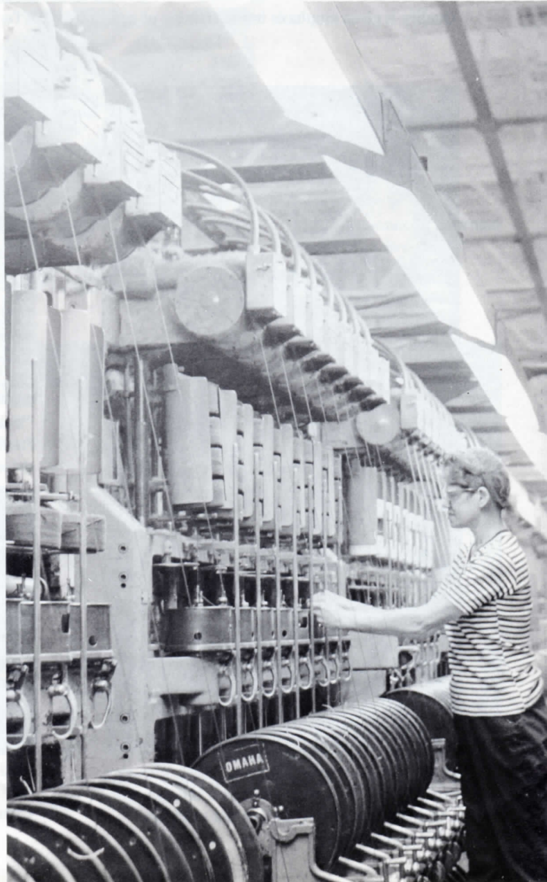
Operations that are mostly machine controlled still require constant attention of operators to get quality. This is June Siefer (252) on the cotton insulating line.
