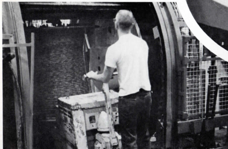
THE COMPLETED CORE truck is removed by means of a hand transport. A fully loaded core might weigh up to 11,000 pounds.
