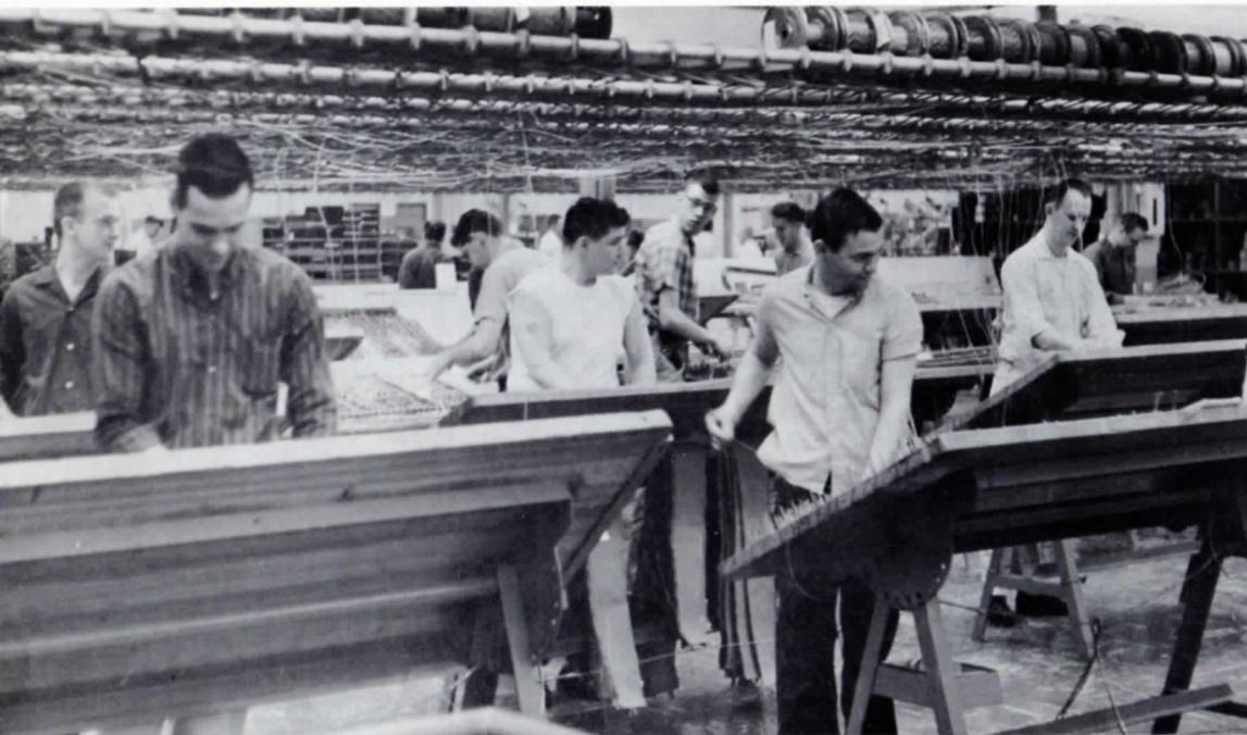
There are several groups who form cables at the Omaha Works. These men (shown above) are forming cables for PBX equipment.
