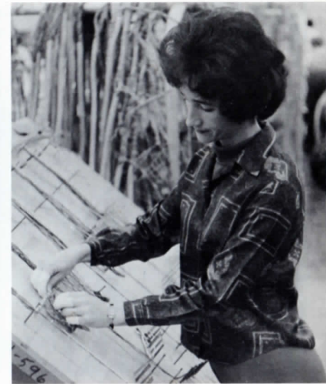
Ellen Leinbach positions wires to form cable.
