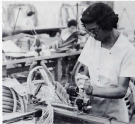
Odessa Bunch skins insulation off wires using a skinning machine.
