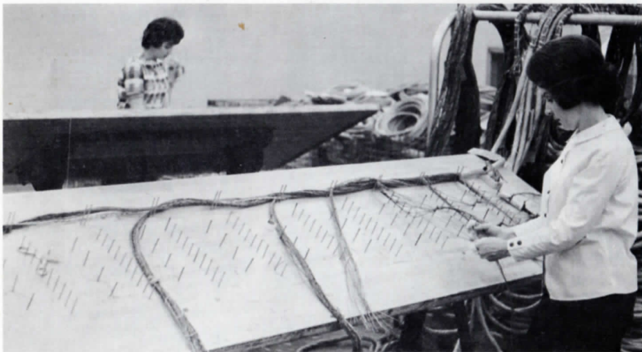
Gladys Stone, (back), and Frances Barnhart form cable to be used in test trunks.
