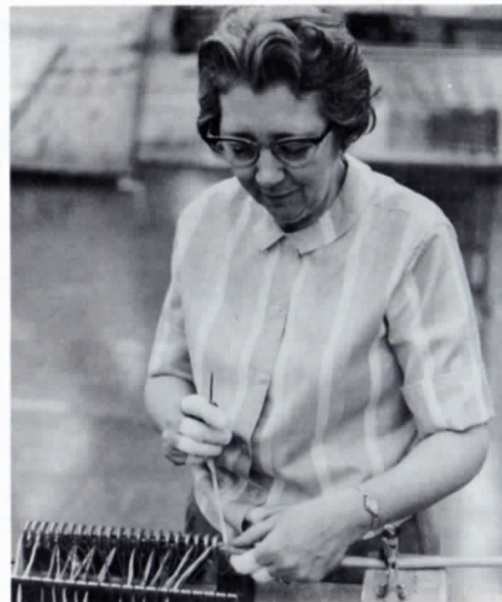
Eletha Beam has become an excellent seamstress when it comes to sewing a cable.
