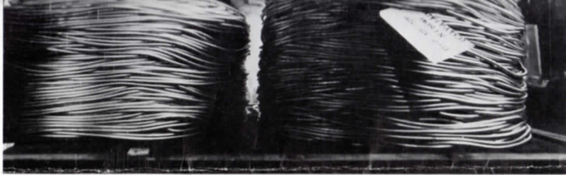
The Bell System's new "activated" solder is formed into coils of 1/4-inch rod on an extruding machine operated by Nassau's John Egnat. Photos by Dave Thomas.
