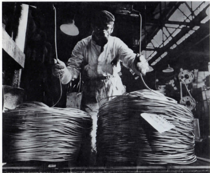
The Bell System's new "activated" solder is formed into coils of 3/4-inch rod on an extruding machine operated by Nassau's John Egnat. Photos by Dave Thomas.
