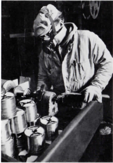
After being drawn into thin wire, solder is wound onto compact spools, ready for shipment to manufacturing and installation points throughout the Bell System. The operator is William Gorman.
