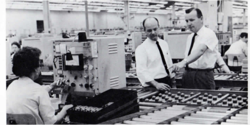
Bob Speights, (731), and Gordon McLean, (751), made a physical rearrangement in the wire spring relay testing and adjusting area which involved conveyors to increase efficiency and production.
